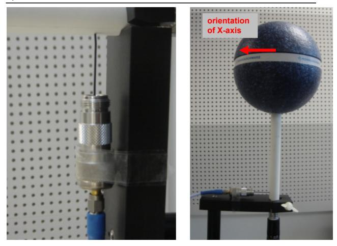
The FSH-screenshots on the next page have been taken with the measurement setup above. The only difference is, that the transducer factors have been applied as described in the next chapter, so that the reading is in  $dB\mu V/m$ .
